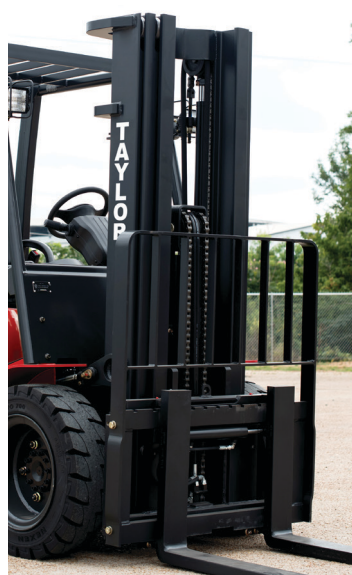
Durable Nested I-beam Design Yields Optimal Visibility
