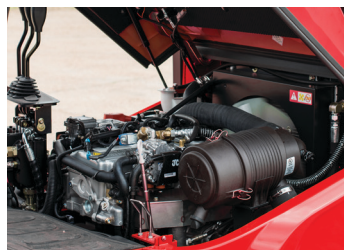
Easy Lift Clamshell Hood (Service & Inspection can be performed from ground level)
