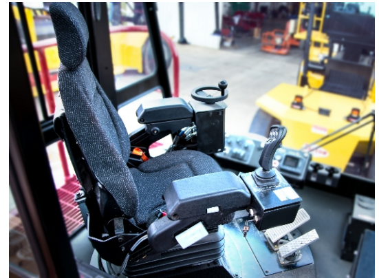
Fully Enclosed 2-door Cab - 180° Rotating Operator Platform (Standard)
