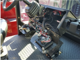
Flip-down Dash with Color/Number Coded Wiring (Standard)
