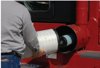
Donaldson Air Cleaner with Safety Element (Standard)
