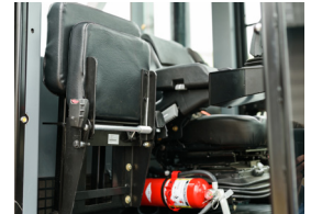
Fully Adjustable Mechanical Seat (Standard)
