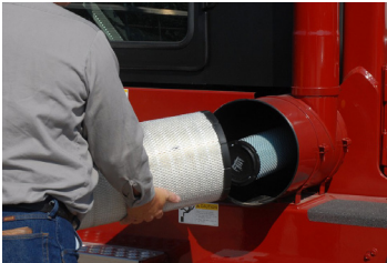
Donaldson Air Cleaner with Safety Element (Standard)
